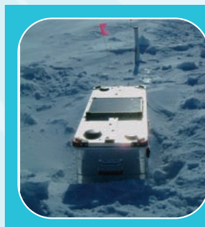
> These ice-buoys carry tiltmeters that may allow the remote measurement of ice thickness. (© D. Mercer, SAMS)
