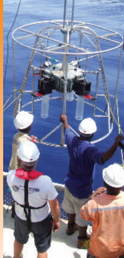
Lowering a sediment corer to collect seabed samples off PNG.
