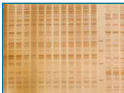
Silver stained polyacrylamide gel demonstrating reproducibility of the method. Virtually identical banding patterns were obtained from different DNA extractions of the algae tested.
