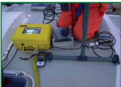
Lightweight stereo video equipment. The yellow case contains two digital camcorders and time code generators. The twin cameras are mounted on the ends of the T bar and the system is powered by a battery in the square grey case.
