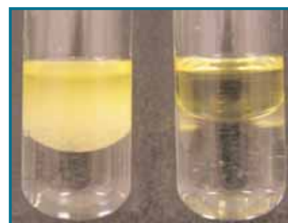
One of our novel emulsifiers mixing olive oil and water (left) alongside its control without emulsifier.
