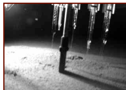
Image of the oxygen and pH electrodes slowly being inserted autonomously into the seabed at 300m depth in the Arabian Sea. These in situ measurements allow us to obtain high resolution oxygen and pH profiles with depth into the sediment without the disturbance created by bringing sediment back to the ship for measurements.
