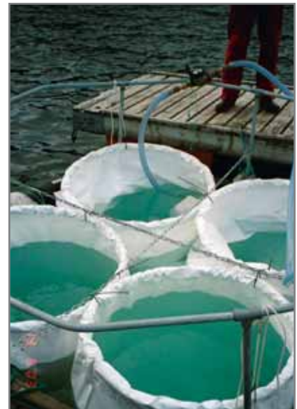
Experimental mesocosms used to test the effect of inorganic and organic nitrogen on planktonic microbial communities (Image: Linda Gilpin)
