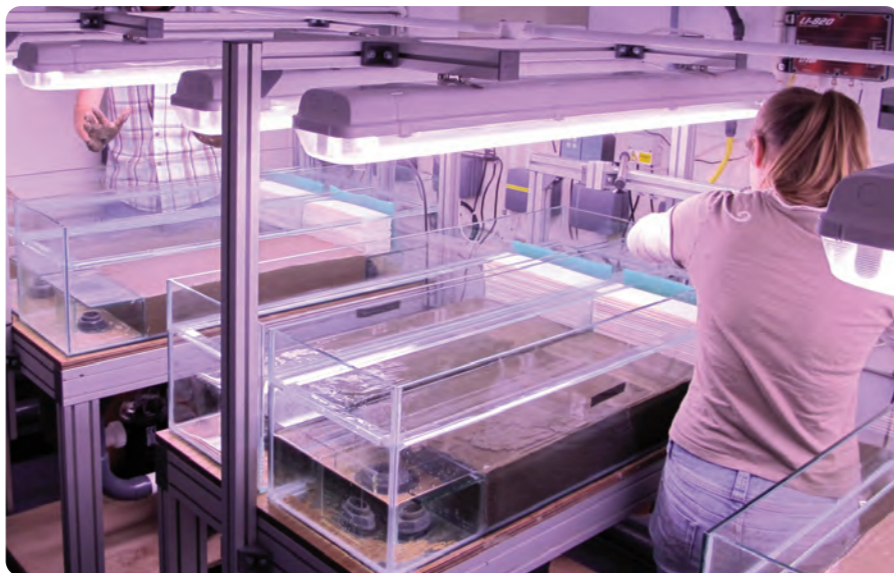
FIGURE 2: Custom built facility with recirculating seawater tanks containing sediments.
