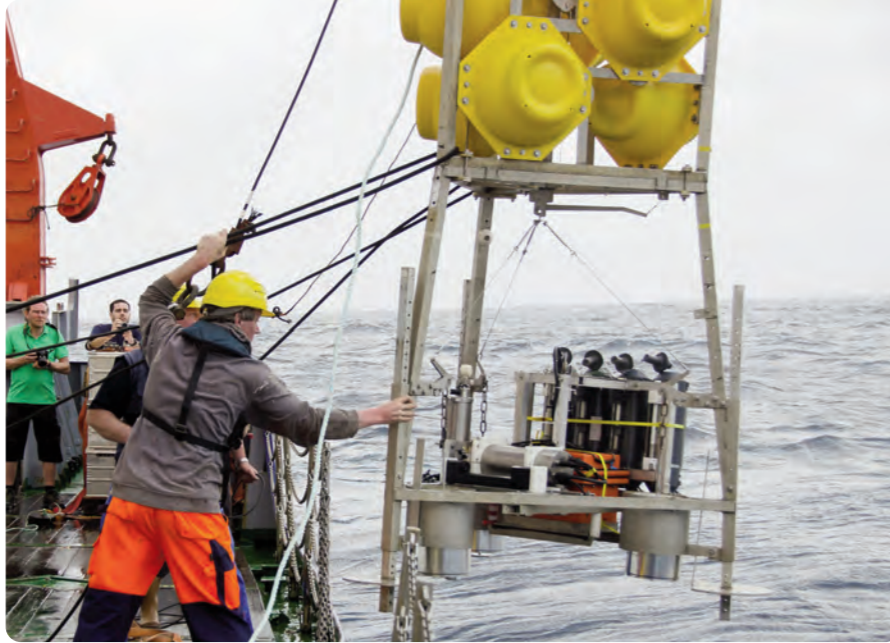
FIGURE 1: Deployment of a SAMS benthic-lander system from RV Poseidon north of Senghor Seamount, February 2013. The lander is equipped with a transmissometer, acoustic current meters and bottles to collect water samples near the seafloor.
