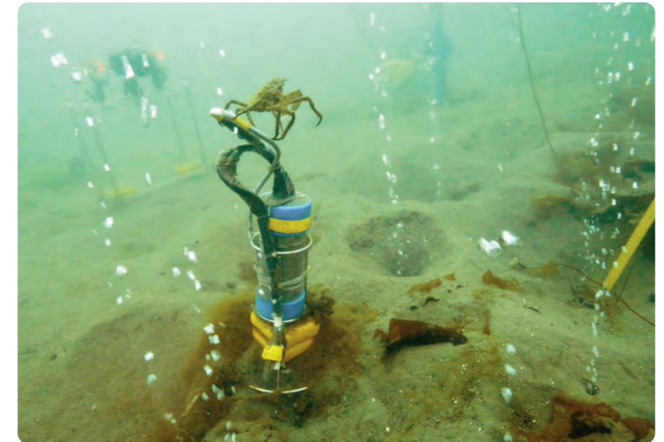
FIGURE 3: Sensor monitoring CO 2 concentrations in the bottom water at the release site.
