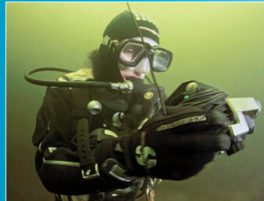
PICTURE 1: NFSD studies have been integrating GPS with dive computers to improve georeferencing underwater.
