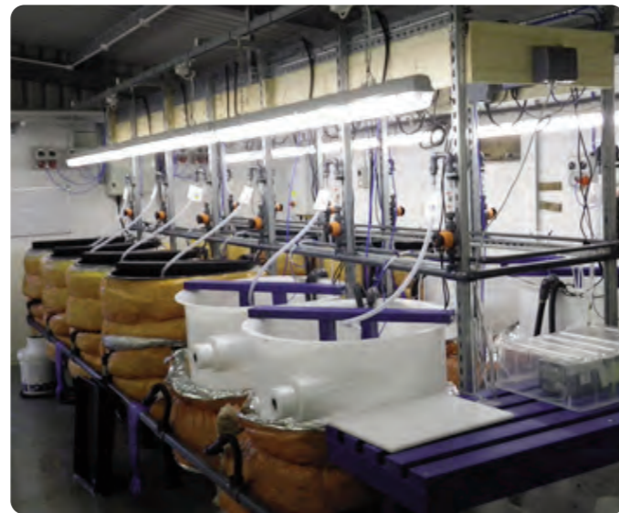
ABOVE: The VOrtex Resuspension Tank (VORT) array in the SAMS Alan Ansell research aquarium: All tanks are lagged to facilitate above ambient temperature; dosing pumps and carboys with chlorine stock below can be seen bottom right.
