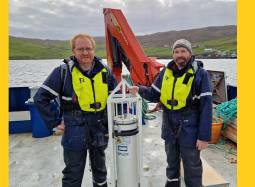
The Imaging FlowCytobot (IFCB) uses a combination of lasers and cameras to detect and photograph microscopic, single-celled phytoplankton in the water, before uploading for specialist data analysis, detection and monitoring.
