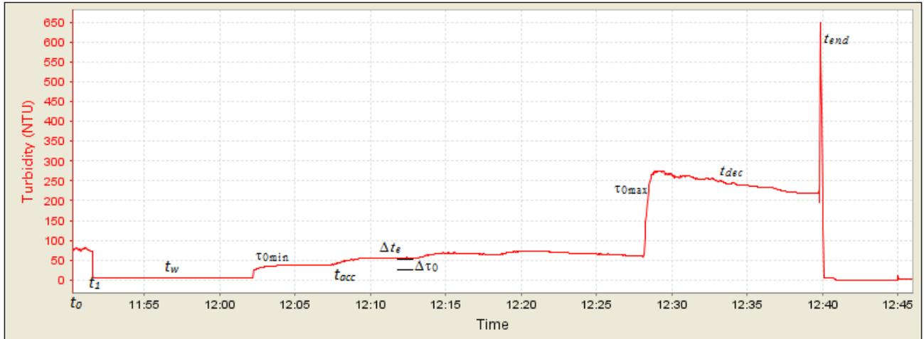
**Figure 4. Example sediment concentration (turbidity) time series showing the various phases of an erosion experiment.**
