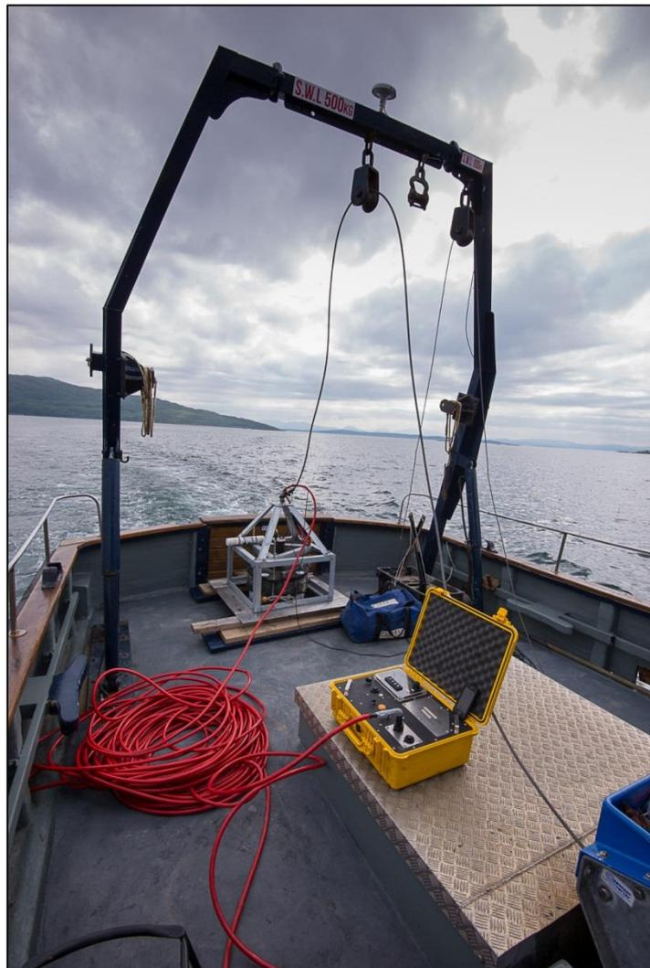
**Figure 6. Voyager I benthic flume, communication/power cable and purpose-built control unit.**
