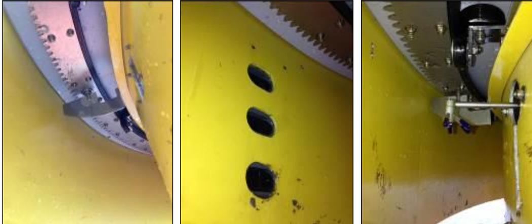
**Figure 3. Photographs showing the paddle (left), the vertical OBS array (middle) and the Nortek Vectrino acoustic current sensor (right).**
